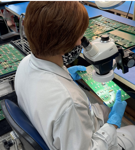
Operators manually inspect assemblies in addition to machine-driven inspections such as automated optical inspection (AOI), X-Ray, and flying probe in-circuit testing.
