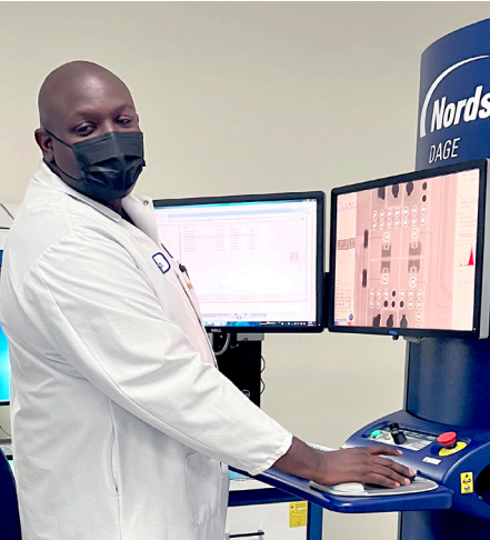
X-Ray inspection allows operators to visualize complex PCBA's they otherwise could not optically inspect. This additional verification process between assembly stages prevents soldering faults and ensures quality and reliability.
